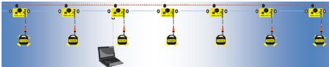
Distributed DAQlink Seismograph System
